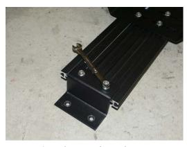
Attach extrusion adapter bracket to 18" section of extrusion using (2) 1/4" x 3/4" bolts and serrated nuts. (7/16" Wrench)
